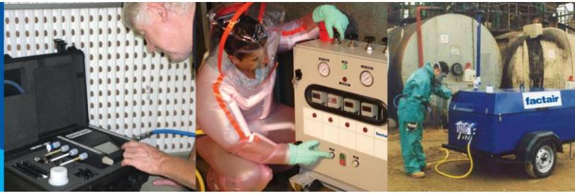
The F2257 breathing-air back-up trolley and the F2257A breathing-air filtration and back-up trolley is to provide breathing quality air from a compressed air supply for up to 2 users wearing positive pressure demand masks. The 3 stage filtration system on the F2257A comprises a pre-filter, coalescing and carbon stage, removing liquid and solid particulate down to a size of 0.01 micron and then oil vapour and odour down to 0.003 p.p.m (exceeding the criteria laid down in BS EN 12021).
